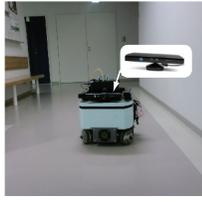
Fig. 5. Mobile robot equipped with four RGB-D cameras (Kinect)
