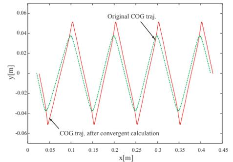
Figure 6: Refined COG trajectories
