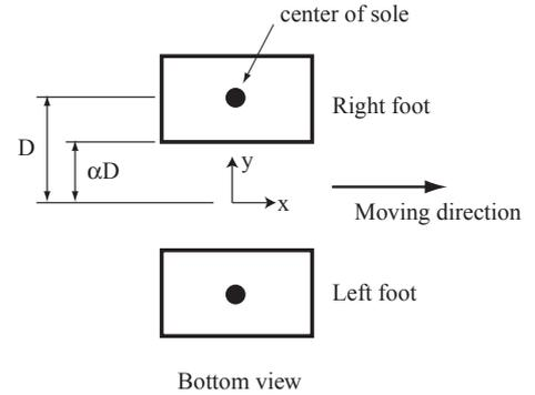
Figure 1: Condition to keep the ZMP in soles
