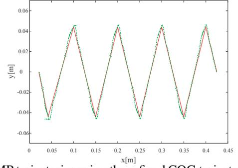
(a) ZMP trajectories using the refined COG trajectory obtained by convergence calculation
