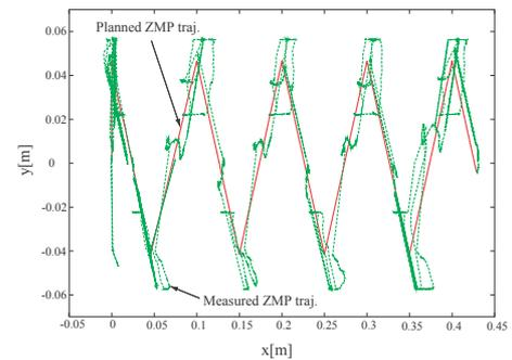
Figure 10: Measured ZMP trajectories
