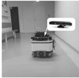
Fig. 6 Mobile robot equipped with RGB-D cameras (Kinect) [29]
